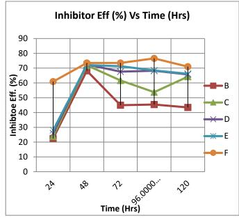
Figure 3.Inhibitor Efficiency (%) Vs (Time hrs)
