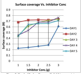
Figure 8. Graph of Surface Coverage Vs Inhibitor conc. (g)
