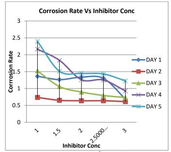
Figure 7. Graph of Corr. rate (mg/cm<sup>2/</sup>yr) Vs Inhibitor conc. (g).
