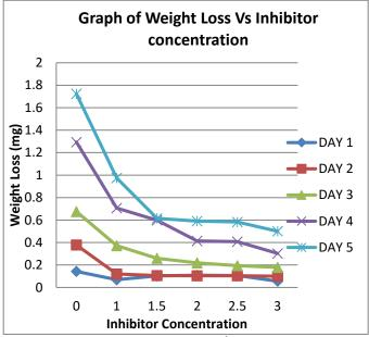
Figure 5. Graph of Weight loss (mg/cm<sup>2</sup>) Vs Inhibitor conc. (g)
